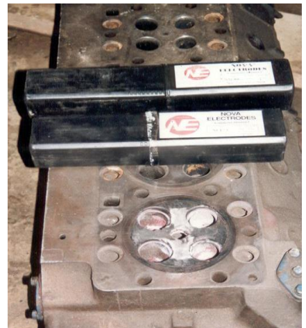
Bulldozer cylinder head (Komatsu) cracked at combustion chamber – repaired by NH 88 and NCI 20 using combustion welding (passed the leak detector test).
